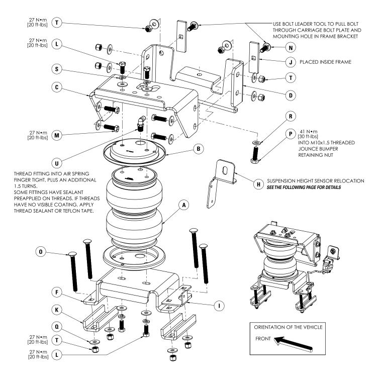
Models equipped with rear suspension height sensors require sensor relocation using relocation brackets listed in the kit contents on page 2. **Relocation brackets are not to be installed if vehicle is not equipped with sensor**
