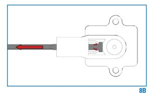
Flip linkage assembly 180°, then insert back into ride height sensor.
