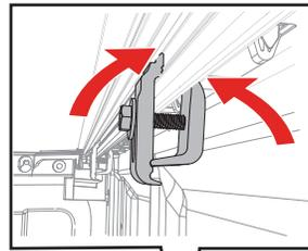
The front/cab end of the side rail has an extension that will sit on top of the truck bed rail. The plastic end cap will be pushed up against the end of the bed brace.
