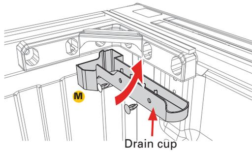
The drain cup (M) has a spout that will be directed into the hole in the side of the truck bed wall. Repeat on the driver's side.
