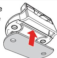
Position the buckle ends (I) with the open side facing the bed cover panel. Use a Phillips screwdriver to install the two buckles into the pre-drilled holes on the front header panel with the provided screws (K) and the nutsert (L) inserted from the backside of the panel. **DO NOT use a screw gun, securely tighten by hand only.**
