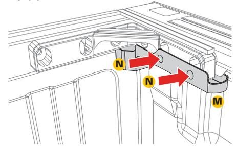
**5** Attach the passenger side rail (C) to the truck bed rail. Note that the side rails are left and right, the prop rods will be on the inside of the bed. Position the clamps (H) as shown, to the front/cab, to the rear/tailgate, and the third in the middle. Tighten the clamps to approx. 10 ft-lbs torque. **Do NOT Overtighten.** Repeat on the opposite side with the driver's side rail (B).
