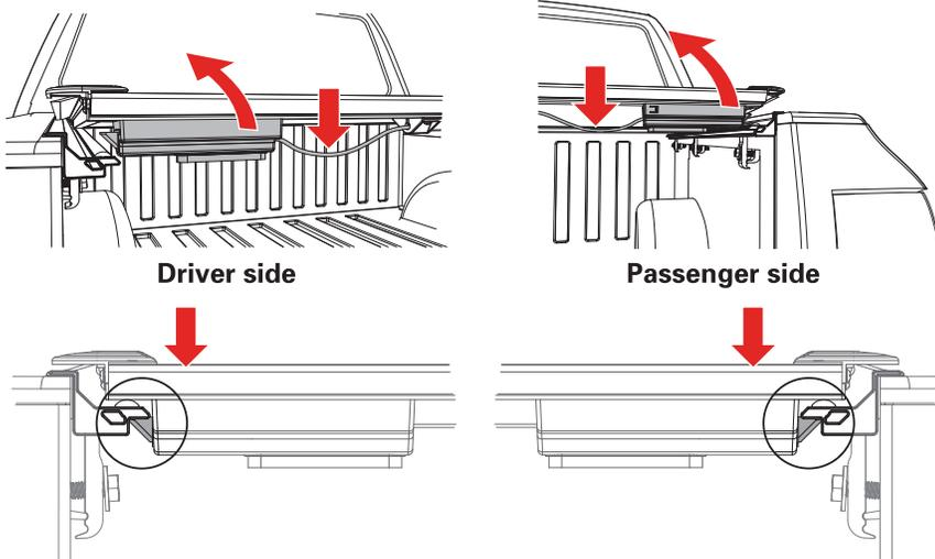
**14** Retighten the cover retainer clamps once the desired fitment is reached. **You are ready to drive with your cover in the closed position.**
