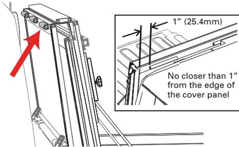
**12** Unfold the cover (A) towards the tailgate. Then confirm each panel is centered side to side and front to back on the truck bed. If adjustments are needed, loosen the cover retainer clamps (G) and shift the cover until positioned correctly. The rear edge of the cover and tailgate seal should rest on top of the tailgate. For proper sealing, the tail panel will overlap by .5".
