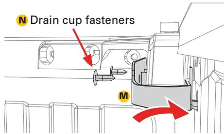
With the drain cups (M) in place, insert the drain cup fastener (N) into each hole in the side of the drain cups. Repeat on the driver's side.
