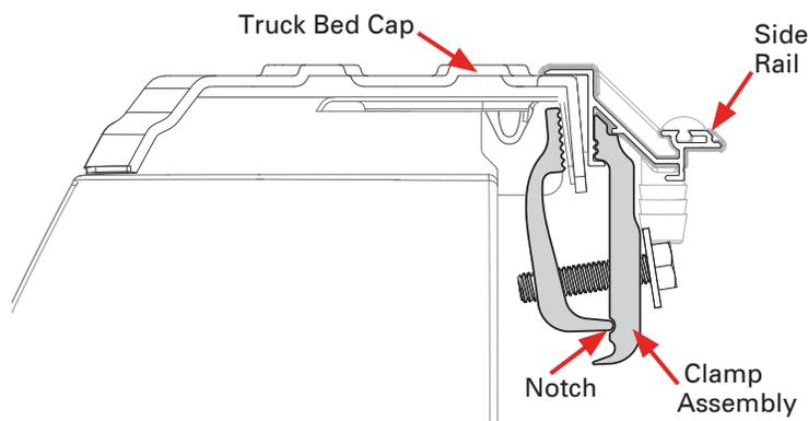
**IMPORTANT:** In order for the cover (A) to operate properly the side rails (B & C) **MUST** be square (90° angle) to the truck bed rails. This allows the rear latch to engage properly.
