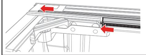
The side rail plastic end cap will drain into the drain cup.
