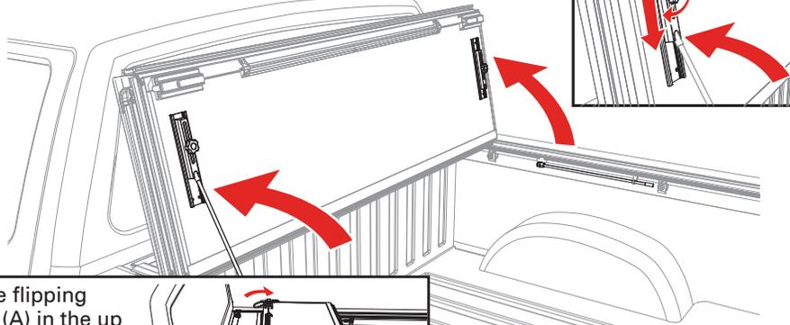
Before flipping cover (A) in the up position make sure to stow the straps using the clips on the underside of the folded cover.
