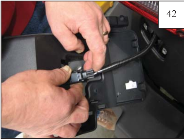
Reconnect light of license plate frame.
