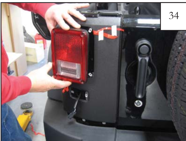
Using a #2 Phillips screwdriver, remove the tail light.
