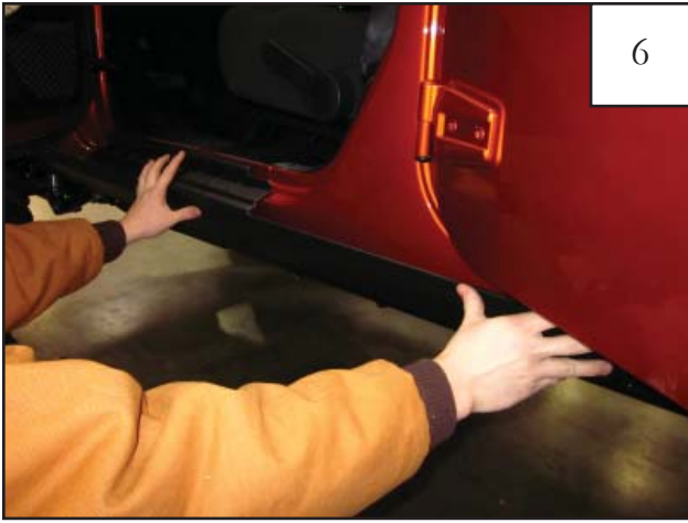
6 Place part on vehicle, making sure to line up edges of part with edges of vehicle and holes in part with clips installed in step 4. Ensure that all tape tabs are accessible.
