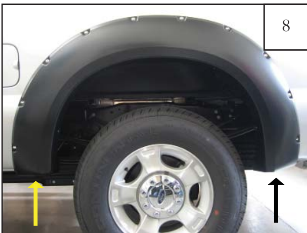
Using a 5/32" Allen Wrench and 3/8" socket, install bolt, Washer (WA1-0010), Spacer (SP1-0008), Washer (WA1-0017), and Nut (NU1-0015) through bottom two holes in flare and into factory holes. See step 9.
