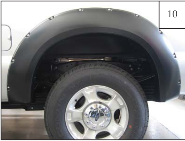
Completed rear flare installation.
