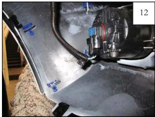
Using a flat head screwdriver, with a pressing motion, remove seven plastic clips located inside of bumper cover. Remove front bumper extension.
