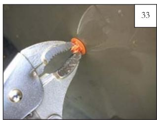
Remove three clips from fender using vise grips, pulling with a rocking motion. See step 34.
