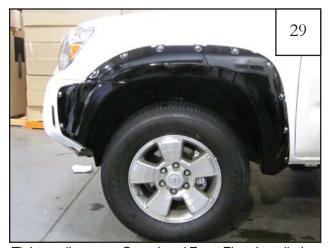
Tighten all screws. Completed Front Flare installation
