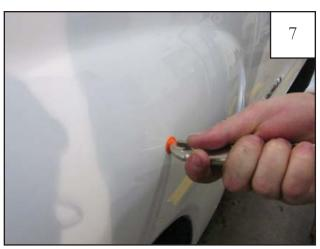
Remove one clip from front using vise grips, pulling with a rocking motion. See step 8.
