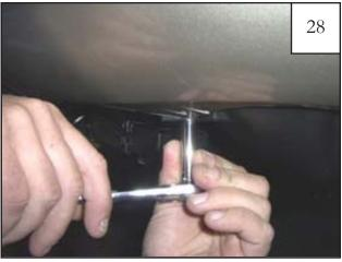
Pull down bumper cover and slide splash shield back in place. Install supplied hex screw (SW1-0036) in front of bumper cover to fasten splash shield to bumper
