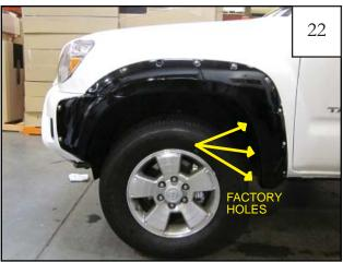
Reposition flare on fender and install three 20mm hex screws (SW1-0036) through holes in flare and into factory holes
