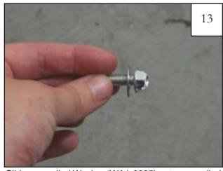
Slide a supplied Washer (WA1-0005) onto a supplied Hexhead Slot Screw (SW1-0005).
