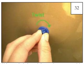
Using a clockwise twisting motion, remove eight factory plastic clips from fender. See step 34.
