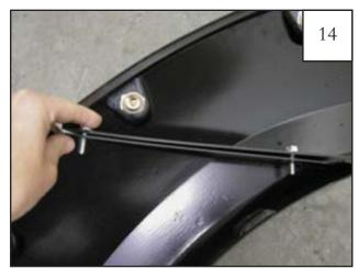
Insert the Screw/Washer assembly through the hole drilled in the end of the Front Main Flare and into the corresponding hole in the Front Bumper Piece. Two places.
