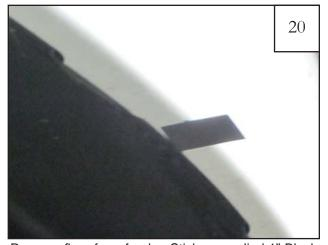
Remove flare from fender. Stick a supplied 1" Black Tab (MT1-0002) over marks made in step 18.
