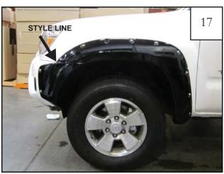
Hold the flare firmly on the fender. Make sure to line up the flare and bumper piece along the style line to ensure correct installation.
