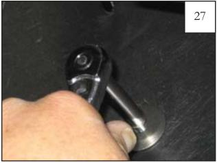
Install a supplied SS Fender Washer (WA1-0015) and supplied 5/16" Nylock Nut (NU1-0019) on back of screws installed in step 27 and tighten. (Note: *Tighten from the back*)
