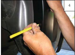
Holding flare in position on fender, use a grease pencil to mark six hole locations. *Note: Rear Flares look very similar. Verify that you have the correct side prior to installation.*
