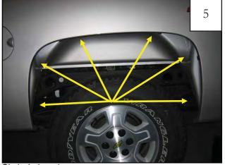
Six hole locations. Note: If fender liner is installed, remove factory tuflocs.
