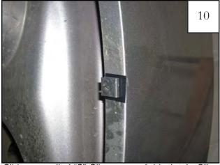
Slide a supplied "S" Clip over each black tab. Clips may need to be adjusted to align with holes in flare. Clips on bottom may need to be pinched in order to stay in position on fender
