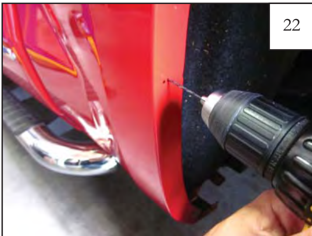
Using a 3/32" drill bit, drill pilot holes at the marks made in Step 20.
