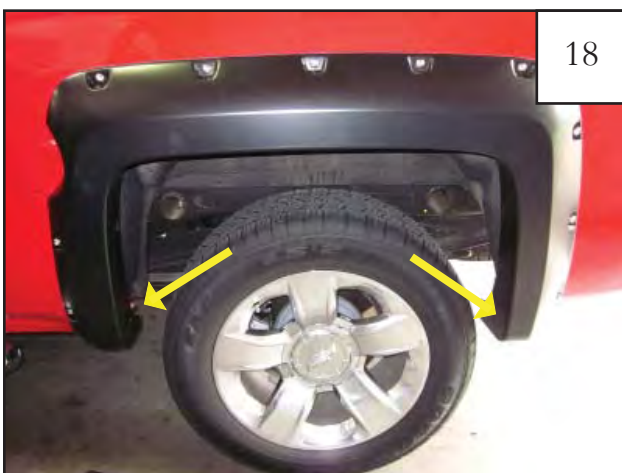
Hold flare firmly in place on fender. Start supplied screw (SW1-0056) at bottom most screw locations (shown). Do not tighten.
