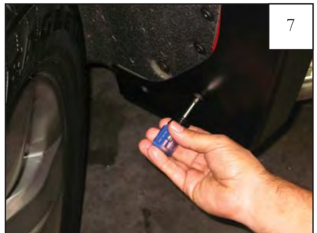
Hold flare in place and start supplied Screws (SW1-0056) through two bottom rear holes in flare and into factory hole in rear of wheel well. Do not tighten.
