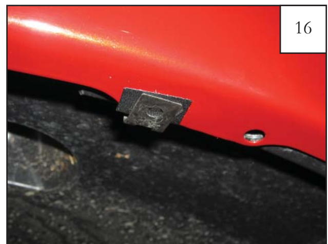
Install #10 U-Clip (CL1-0022) over tab and existing factory hole.
