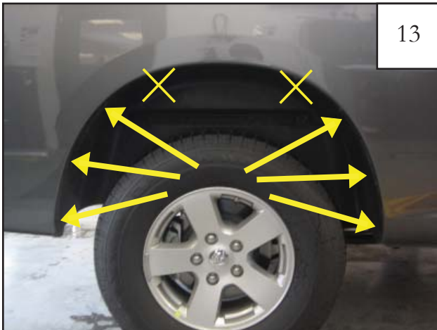
Remove six factory installed screws using an 8mm socket wrench. X's indicate a factory screw that will not be removed.
