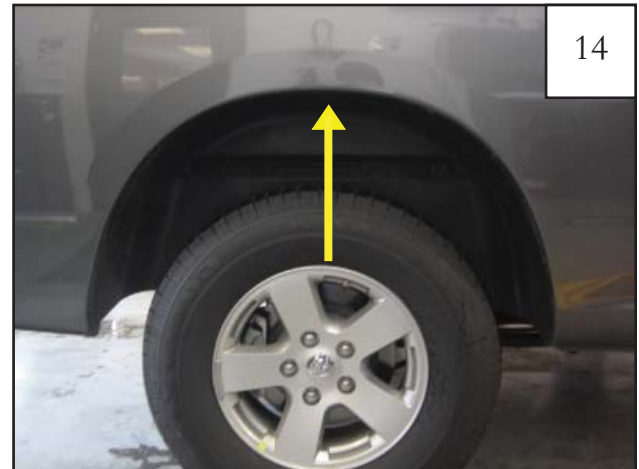
Install #10 U-Clip in this location. See steps 15 & 16.
