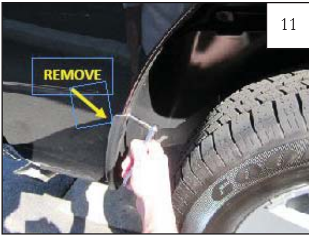
2012 Models Only (Optional): If you encounter a fit problem, remove inner piece at bottom rear and front of wheel well.
