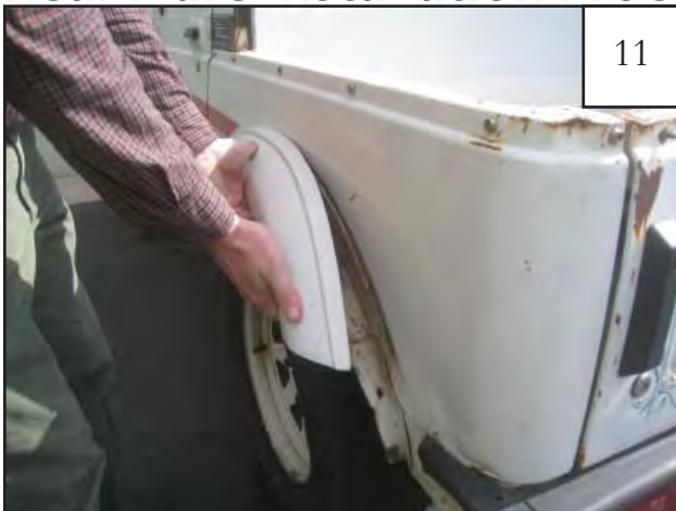
Starting at rear of factory flare, pull up then out on flare to pop it off the metal lip. This will pull plastic rivets from the holes in factory flare. If rivets do not come out, remove them.
