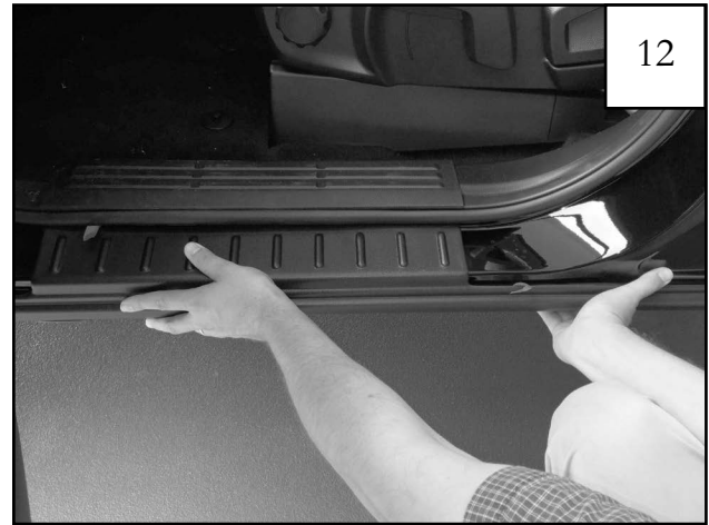
Place part on vehicle, making sure to line up edges of part with edges of vehicle. Ensure that all tape tabs are accessible. Firmly press on exposed areas of tape to tack Trail Armor in place. NOTE: Refer to step 1 for placement of certain tabs.
