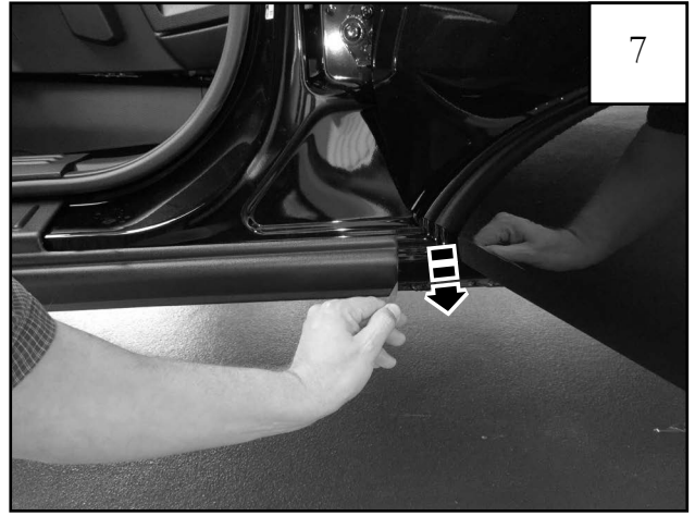
Pull tape liner tab 4. NOTE: Refer to step 1 for additional tape tab identification.
