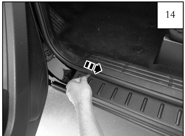
Pull tape liner tab 3.
