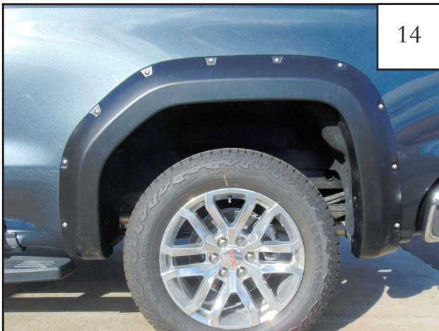
Fully tighten all fasteners, then replace the rear wheel as instructed in your user's manual.
