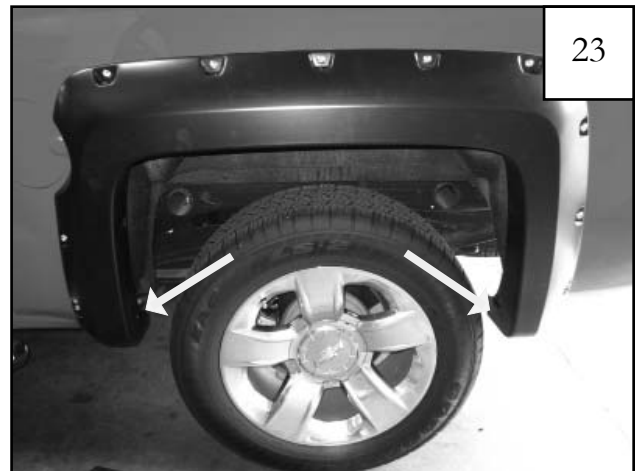
Install supplied screws (SW1-0056) into two lower most holes.
