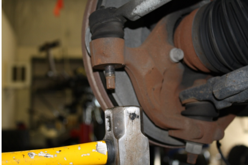
Figure 1: remove outer tie rod end from spindle
