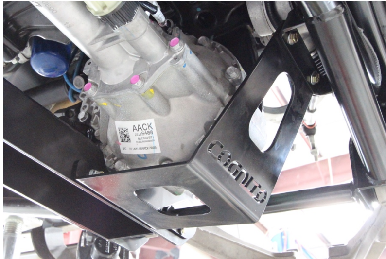
Figure 21: install 1860 skid plate
