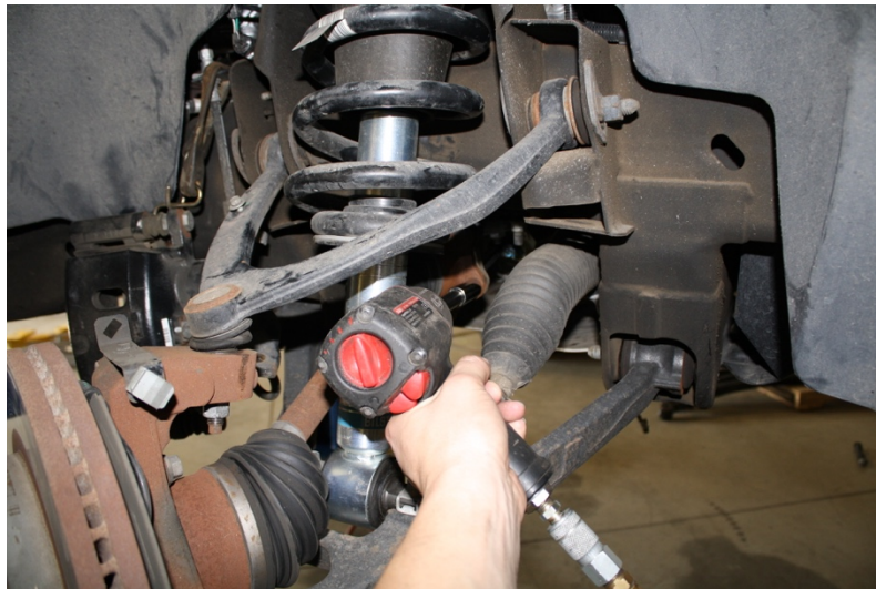
Figure 2: unbolt CV axle from differential
