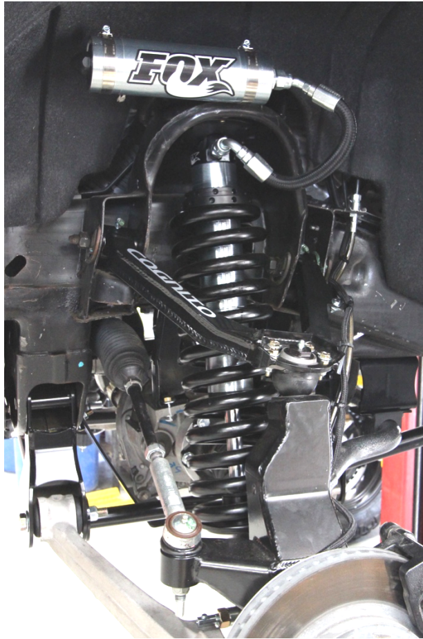
Figure 22: Fox remote reservoir shock mounting
