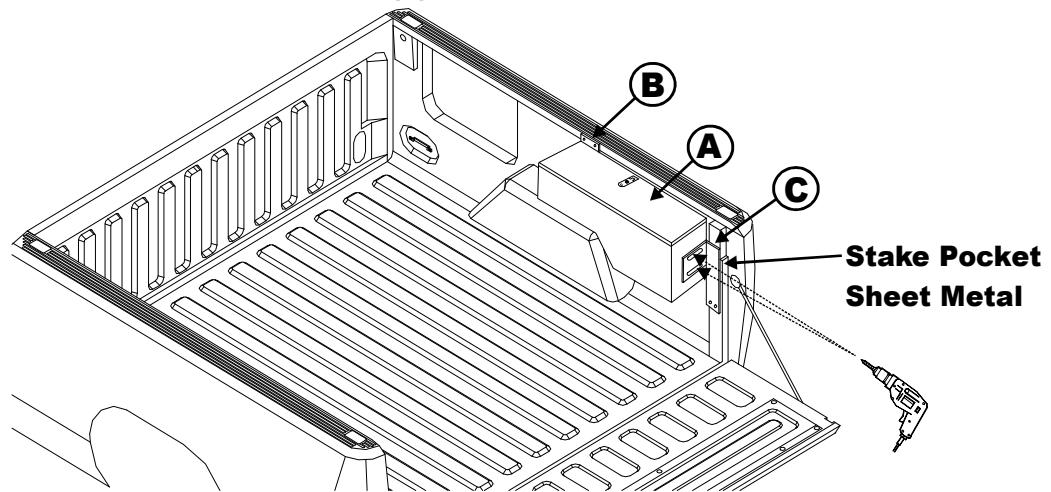
**14****Mounting bracket (C) installation - (1994 - Current) Dodge Ram Pickup beds:**
