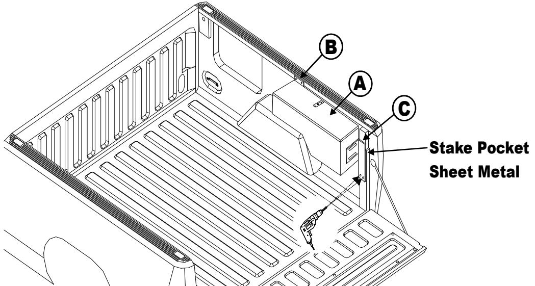
**16****Mounting bracket (C) installation - (1994 - Current) Dodge Ram Pickup beds:**
