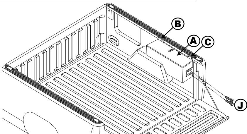
**13****Mounting bracket (C) installation - (1994 - Current) Dodge Ram Pickup beds:**
