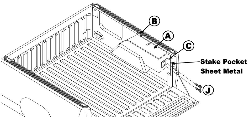
**15****Mounting bracket (C) installation - (1994 - Current) Dodge Ram Pickup beds:**
