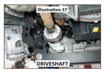
59. Install the new adapter and the new vent hose to the differential vent hose then attach to differential.
