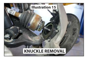
23. Secure the axle up and out of the way so it will not be hanging and over-extend in next steps.
