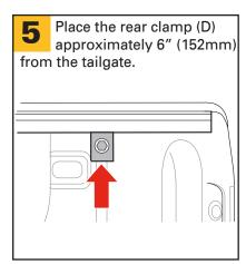
Tighten the clamps (D) starting with the middle, then the front and rear. Always apply downward pressure to the rail when tightening to ensure that the rail sits flush and seals properly. Repeat steps 2 - 6 for the driver side rail (B). 10 ft-lb
