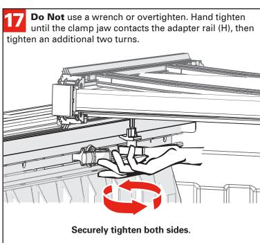
The tethers come installed looped over the bed cover bow with a clamp at the other end. Install the clamp end by sliding the clamp onto the adapter rail (H). Make sure the clamp is positioned as far up onto the rail as possible. Firmly hand tighten the knobs. Install the tethers on both sides of the cover.
