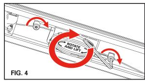
Double-check that the cover is secure and tight to the truck bed by gently lifting the corners to ensure the mechanisms are engaged.
