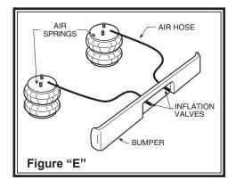
line tubing should not be bent or curved sharply as it may buckle with time. Secure the tubing in place with the nylon ties provided. Push the end of the air line tubing into the inflation valve as far as possible. See Figures "D" & "E".
