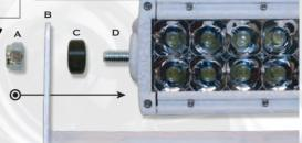
WHETHER MOUNTING THE LIGHT WITH PROVIDED BRACKETS OR BY OTHER MEANS, BE SURE TO USE THE COMPRESSION SPACER. FAILURE TO DO SO WILL CAUSE YOUR LIGHT TO ROTATE OR SPIN. TO INSTALL WITH PROVIDED BRACKETS, REMOVE NUT ON END BOLT AND SLIDE BRACKET ON COVERING COMPRESSION SPACER. REPLACE NUT ONTO END BOLT AND SNUG DOWN. WAIT TO SECURE BOTH NUTS UNTIL YOU HAVE YOUR LIGHT WORKING AND IN DESIRED POSITION.
