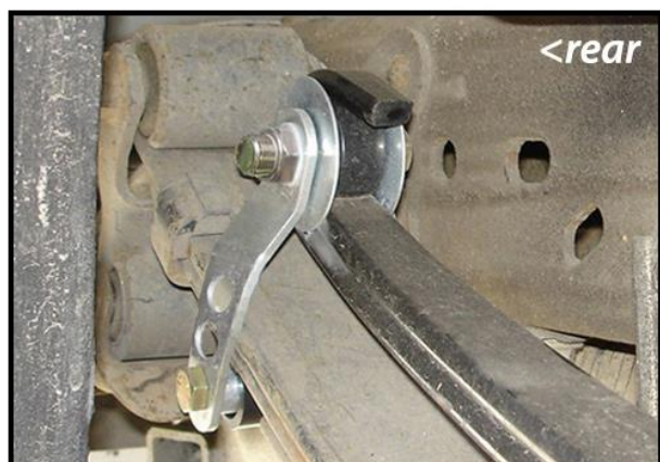
Adjustable pre-load and ride height [fnt/rear]
