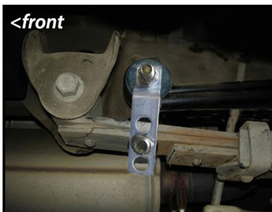
Adjustable pre-load and ride height [fnt/rear]
