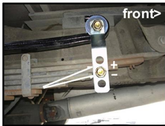
front> Spring preload & ride height
